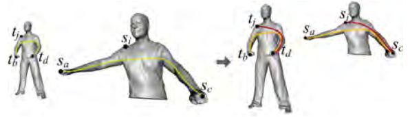
Figure 3: Demonstration of the distortion measure with normalized geodesics defined in (4). Suppose that sample sets S and T each contains three surface points to be matched. The geodesics used in computation of d_{\text{iso}}^{(2)}(s_i, t_j) (red paths on the right) are normalized w.r.t. the local maximum geodesics (yellow paths on the left).
