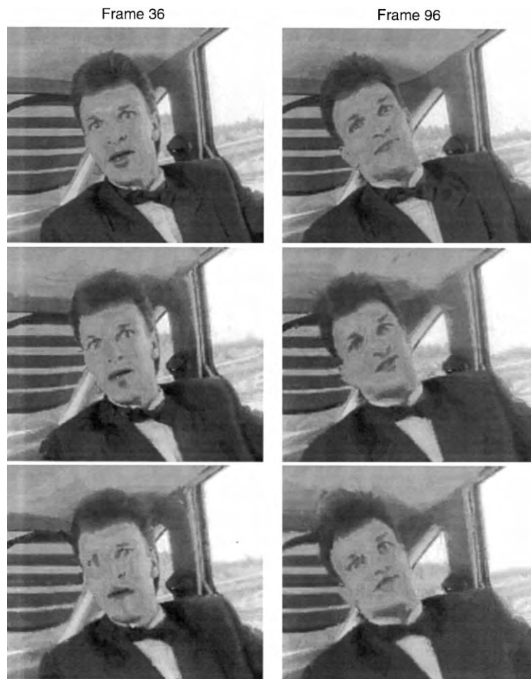
Fig. 13. Coder performance for Carphone sequence at different bit-rates. In the order from top to down, original frames and coded frames at 79 and 50 kbit/s, respectively.
