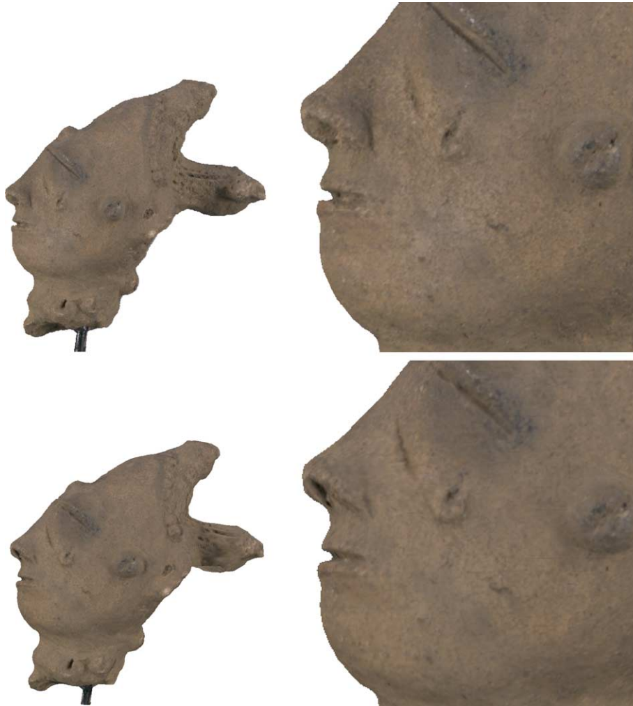
Fig. 23. Textured Anyi model at resolution R=9 (top) and the corresponding image of the sequence masked with the silhouette (bottom); (right) we zoom on the object to observe the high resolution reconstruction performance as compared to the original image.
