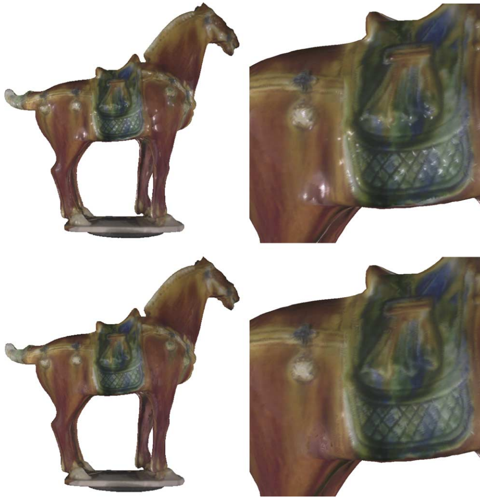
Fig. 19. 3D color horse model at resolution R=7 as a whole (left) and zoomed (right). The surface has been textured by two optimal images, (top) without and (bottom) with highlight elimination. Observe that highlights are spread throughout the surface resulting in a disturbing unrealistic diffuse texture if they are not taken into account during the texturing process.
