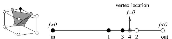
Fig. 11. A marching octree cube and dichotomic subdivision process to find the exact vertex locations of the triangulation.
