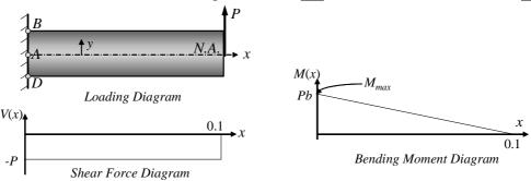
From the shear force and bending moment diagrams, one can identify that the shear force is uniform along the shaft with V=P=18000N, and the maximum bending moment occurs at the section ABCD with a magnitude of  $M_{max} = Pb=18000\times0.1=1800Nm$ . So the *critical* section is ABCD.
