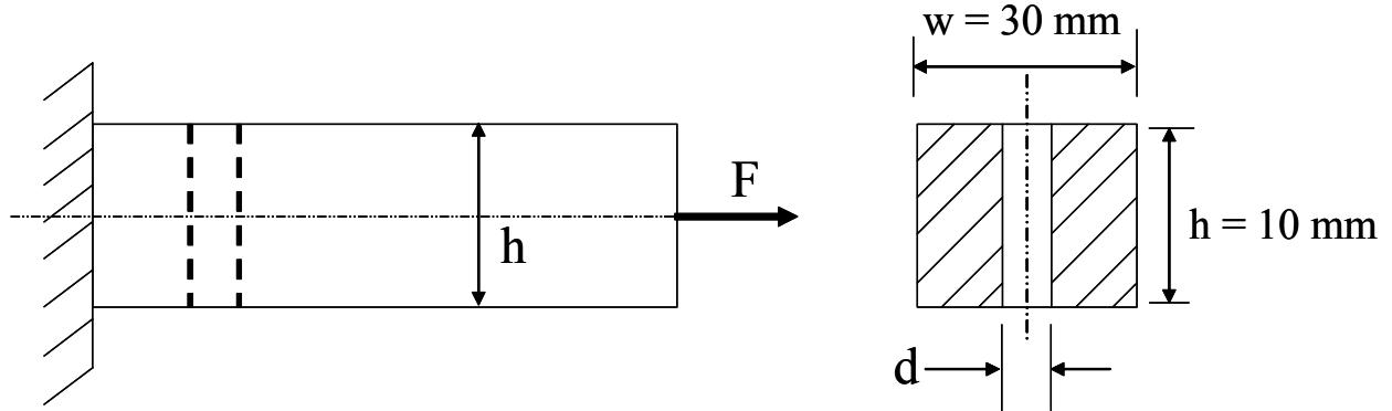
Critical section of the beam is at the transverse hole due to stress concentration at this point. First, we calculate the correction factors:
