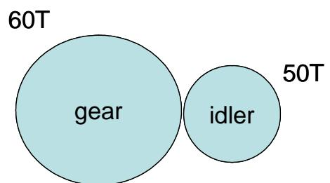
Note: The idler has a slightly different J factor when considered to be the “gear” in mesh with the smaller pinion (0.42) than when considered to be the “pinion” in mesh with the larger gear (0.43).
