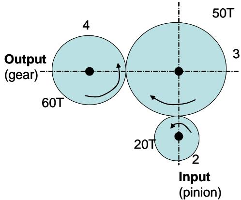
**Problem:** Pinion 2 is shown in the figure runs at 1750 rpm and transmits 2.5 kW to idler gear 3. The teeth are cut on the  $20^0$  full-depth system and have a module of  $m = 2.5 \text{ mm}$ .
