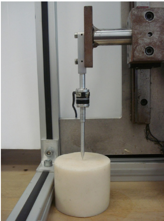
Fig. 13. The cylindrical silicone sample tested in the validation experiments.
