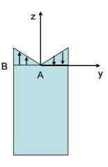
Normal stress due to the bending moment about the y-axis = 0
