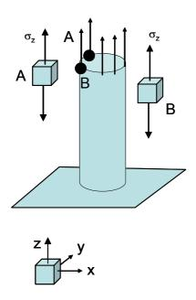
Normal stress due to the bending moment about the x-axis = 0
