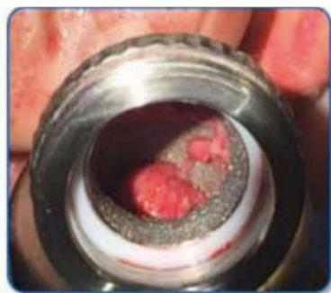
Figure 1. Pump thrombosis in a left ventricular assist device.
