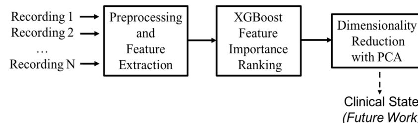
Figure 4. Acoustical analysis block diagram.
