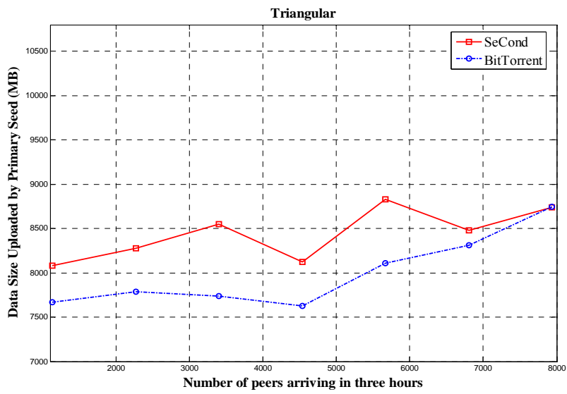
Figure 18. Load imposed on the primary seed for triangular arrival pattern vs. system size
